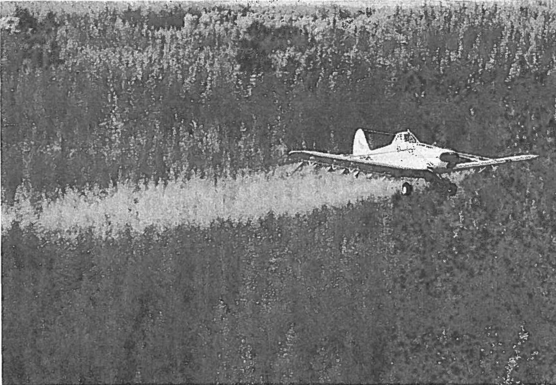
Fig. 2 Piper Pawnee 235B During Application of DDT in the Spruce Woods Provincial Forest.
